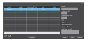
Step 3: When using the mouse to draw a straight line on the micrometer image and setting the scale length, selecting a longer scale length will give more accurate results. For example, selecting 10 small scale lengths will give you more accuracy than selecting only 1 scale length. After releasing the mouse, the image value of the line drawn with the mouse will be automatically updated in the "Benchmark" of the calibration table, as shown in the following figure.
